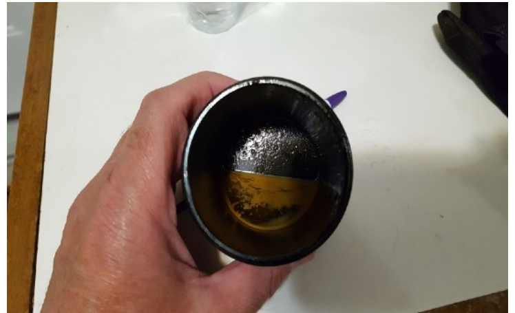
Fig. 3 – Accumulation in catch can after one week at the Tail of the Dragon.
